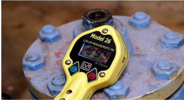
When conducting field surveys looking for contamination in the environment we used a NaI scintillation detector paired with a Ludlum Model 2350 Datalogging Survey Meter and a Ludlum Model 26 Integrated Pancake Frisker. Both of these units were calibrated to measure radioactive interactions in counts per minute.
